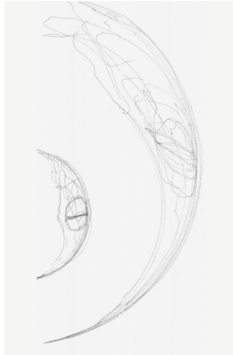
Arm extension drawing apparatus. Maximum reach of just over twelve feet. Its elbow joint allows for more varied and controlled movement. A pen is placed at the hand and at the outer limit of the structure. The duplication is not exact due to inherent distortion resulting from the device's geometry and the amplification of imprecision at the farthest extent.
